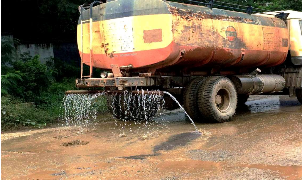
Photograph showing water sprinkling in haul road
